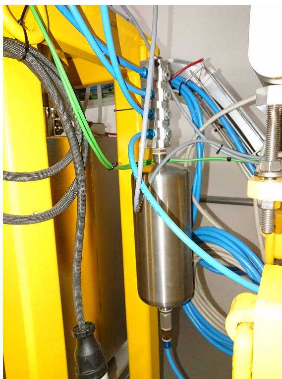
Pic. 3. Buffer tank with a check valve and a local manifold
